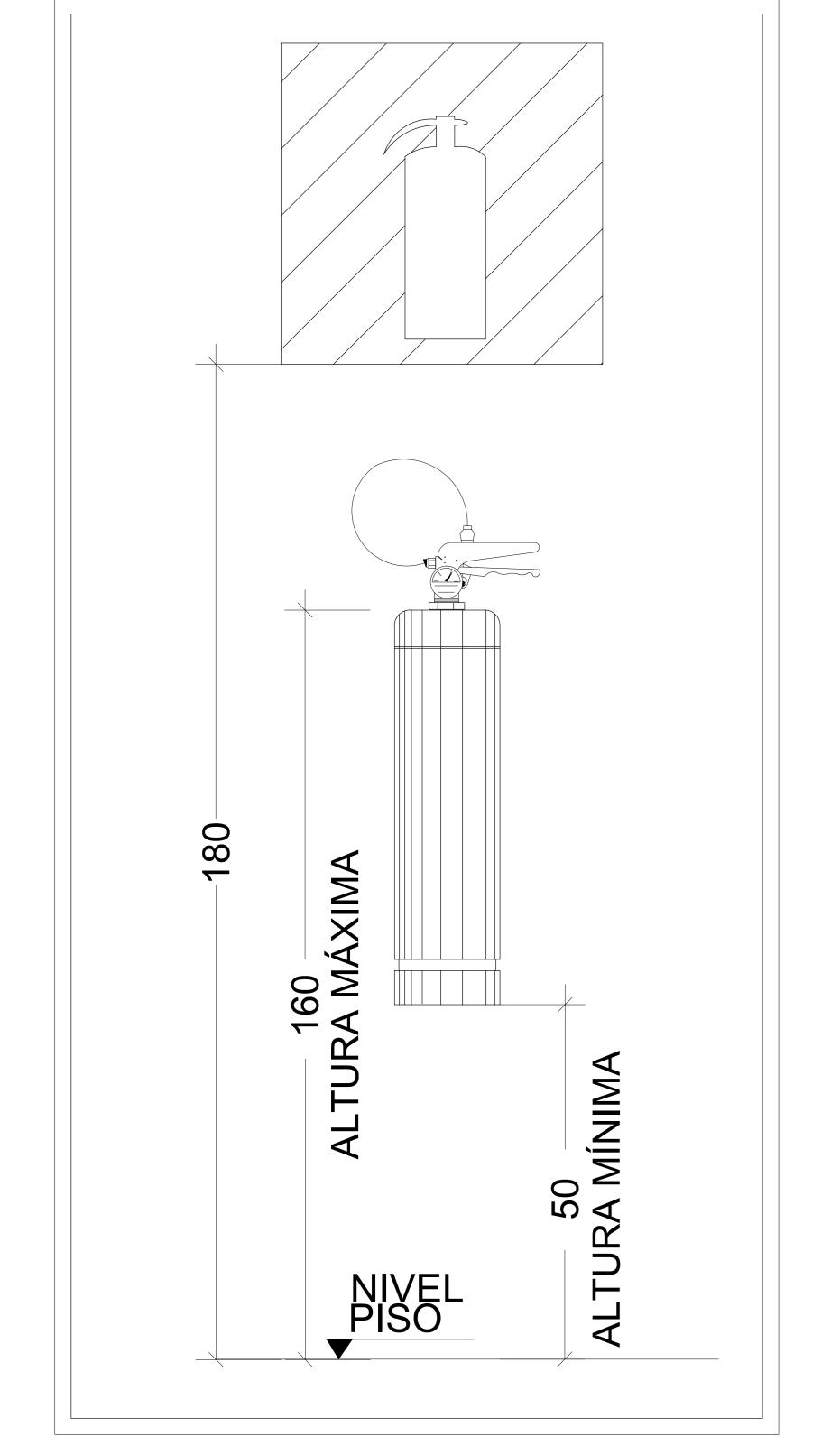
DETALHE EXTINTOR OBS: SEM ESCALA
